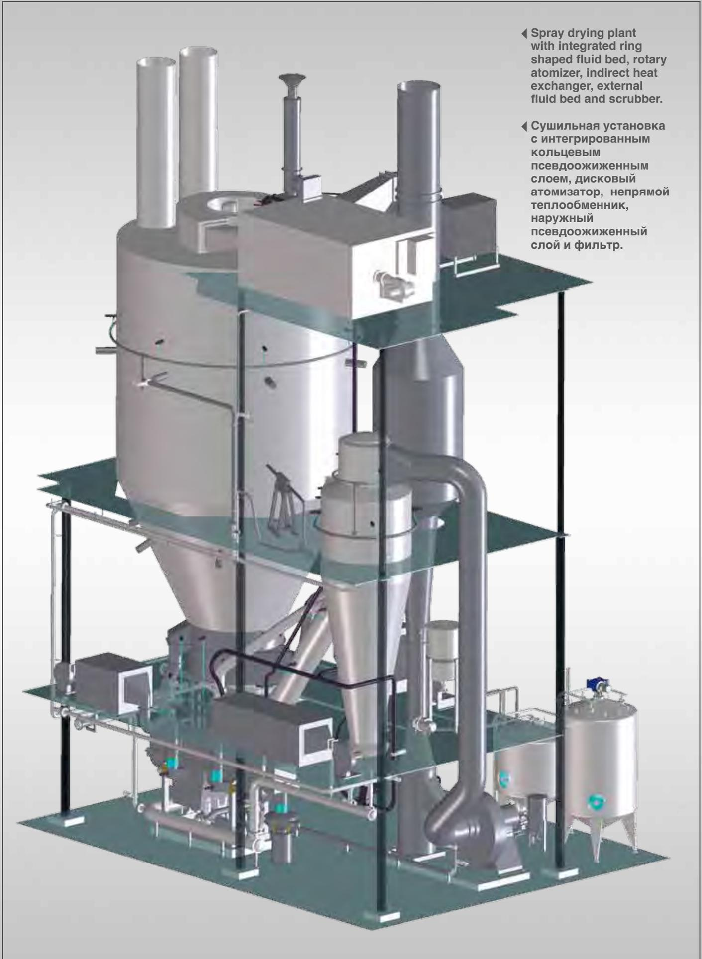
◀ Spray drying plant with integrated ring shaped fluid bed, rotary atomizer, indirect heat exchanger, external fluid bed and scrubber.
